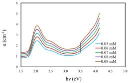
Fig. 5 The absorption coefficient ( $\alpha$ ) of the Celestin Blue B dye - doped polymer film versus the incident photon energy (hv), for different dye concentrations
