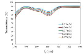
Fig. 3 UV-Vis transmittance spectra of the Celestin Blue B dye – doped polymer films at different dye concentrations
