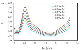
Fig. 9 The imaginary part of the dielectric constant ( $\epsilon_i$ ) versus the incident photon energy (h v) for the Celestin Blue B dye-doped polymer films at different dye concentrations
