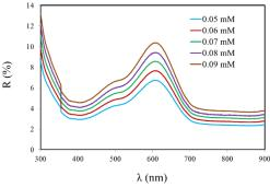
Fig. 4 UV - Vis reflectance (R) spectra of the Celestin Blue B dye – doped polymer films at different dye concentrations
