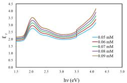
Fig. 8 The real part of the dielectric constant ( $\epsilon_r$ ) versus the incident photon energy (h v) for the Celestin Blue B dye - doped polymer films at different dye concentrations
