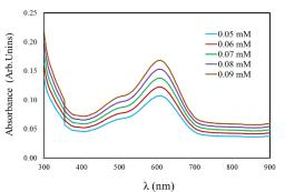
Fig. 2 UV - Vis absorbance spectra of the Celestin Blue B dye – doped polymer films at different dye concentrations
