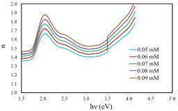
Fig. 7 The refractive index (n) of the Celestin Blue B dye - doped polymer film versus the incident photon energy (hv), for different dye concentrations
